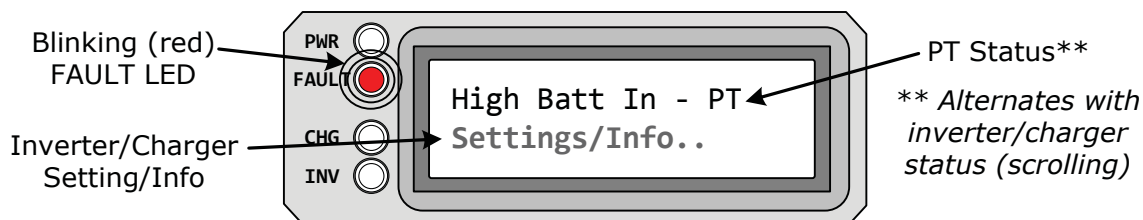
Figure 10-9, PT Controller Fault Message (Example)
