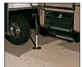
The exclusive StepUp, power 4-step entry, is a revolutionary feature that provides added stability in the step, push button control for easy set-up, and eliminates the inconvenience of wrestling the conventional entry steps in/out every time you travel. The powerful twin motors extend/retract the step in seconds and with all the extra welds we have eliminated the "sag" effect seen on other 4-step entry's.
