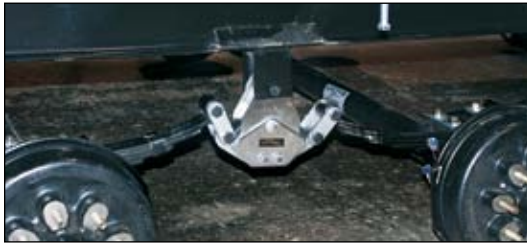
TrailAir® EquaFlex Suspension is standard. Kodiak Disc Brake Package, that includes 8000 lb capacity axles, is available as an option.
