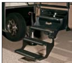
The exclusive StepUp, power 4-step entry, is a revolutionary feature that provides added stability in the step, push button control for easy set-up, and eliminates the inconvenience of wrestling the conventional entry steps in/out every time you travel. The powerful twin motors extend/retract the step in seconds and with all the extra welds we have eliminated the "sag" effect seen on other 4-step entry's.
