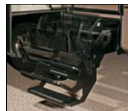
The exclusive StepUp, power 4-step entry, is a revolutionary feature that provides added stability in the step, push button control for easy set-up, and eliminates the inconvenience of wrestling the conventional entry steps in/out every time you travel. The powerful twin motors extend/retract the step in seconds and with all the extra welds we have eliminated the "sag" effect seen on other 4-step entry's.
