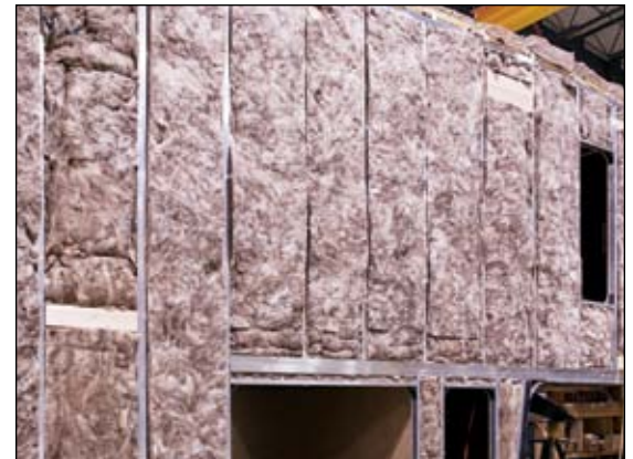
The coach and slide outs have aluminum wall studs and roof trusses positioned 16" on-centers, and the aluminum sub-floor joists are 14" on-center. Residential style high density wool insulation, in the side walls, is glued into place to prevent future settling. All spaces and voids are filled with wool insulation as well.
