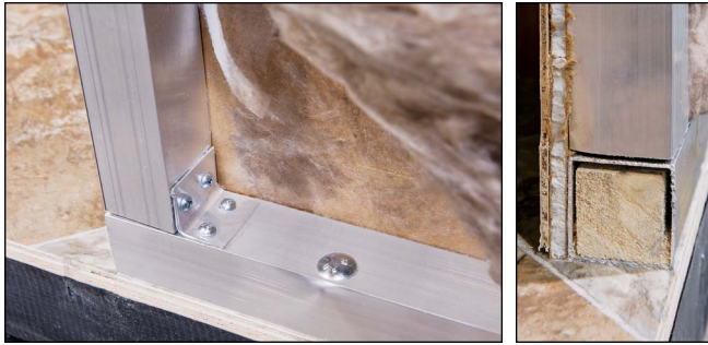
All aluminum sills and wall studs are mechanically joined and the aluminum sill tubing is fully reinforced internally with wood, providing greater strength and stability when it is "bolted-through", never screwed, to the sub-floor structure and the steel frame below.
