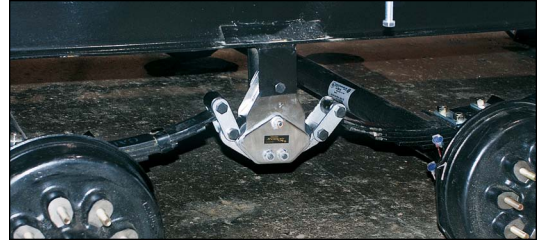
TrailAir® EquaFlex Suspension is standard. Kodiak Disc Brake Package, that includes 8000 lb capacity axles, is available as an option.
